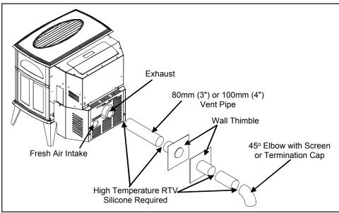
Figure 9: Straight through wall Installation.
